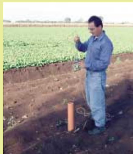
Regular water table tests for nitrate or pesticide leaching are carried out through pipes 2m deep. Here a fieldsman is taking samples to monitor the water quality beneath a spinach field.
