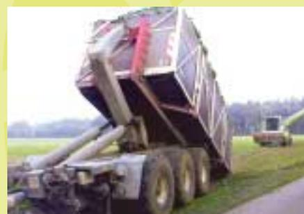
The specific development of wide anti-compaction tracks on harvesting equipment has done much to minimise the effect of heavy machinery on spinach fields (top). Separating field and road transport (above) also helps to minimise the impact on fields - the high tyre pressures necessary for road use are damaging to soil fertility.
