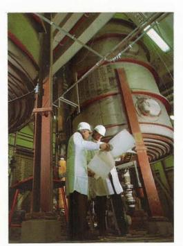
These semi-continuous edible oil deodorisers are part of a new oil processing department at Van den Bergh en Jurgens margarine factory at Nassaukade, Rotterdam, in the Netherlands. The equipment, which incorporates advanced automation, will give energy savings.
